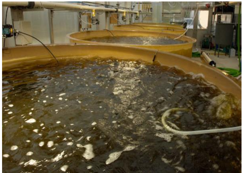
The photo below shows tanks hatcheries use to grow algae they feed to larval and juvenile shellfish.
